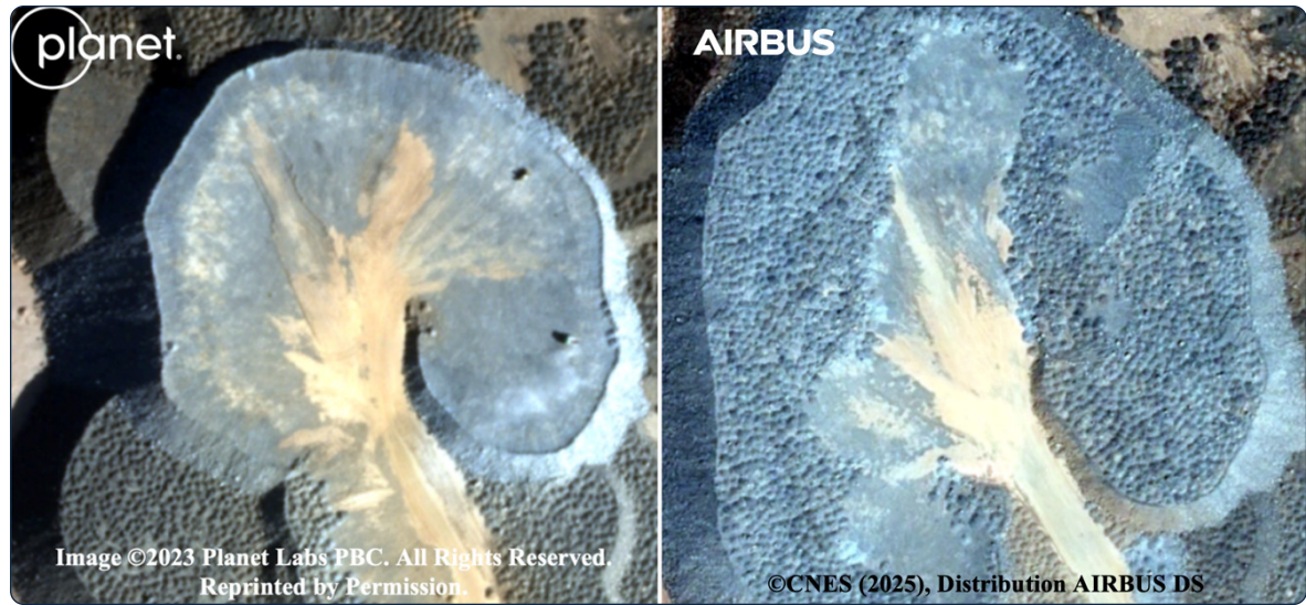
Figure 2: Satellite imagery displaying earth movements at the Alliance for Mining site, November 2023 (left) and March 2024 (right). These include both large-scale movements of overburden rock/tailings (pictured), as well as the collection of small piles of what is presumably ore-bearing rock destined for downstream refining.
