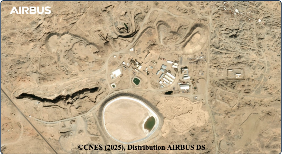
Figure 17: Satellite imagery of the Delgo Mining site, December 2024. The site is located in Sudan's Northern State. The site has several small open-pit mines, alongside ore heaps and tailings mounds. It also has an area for refining, including a holding pond, leach heaps, and leach ponds.
