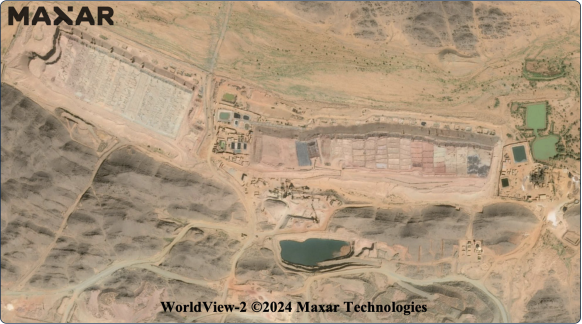
Figure 9: Satellite imagery of the northern portion of the Ariab Mining Company site, December 2024. The site is located in Sudan's River Nile State. The site has a large open-pit mine, along with areas for refining, including holding ponds, leach heaps, and chemical storage tanks.
