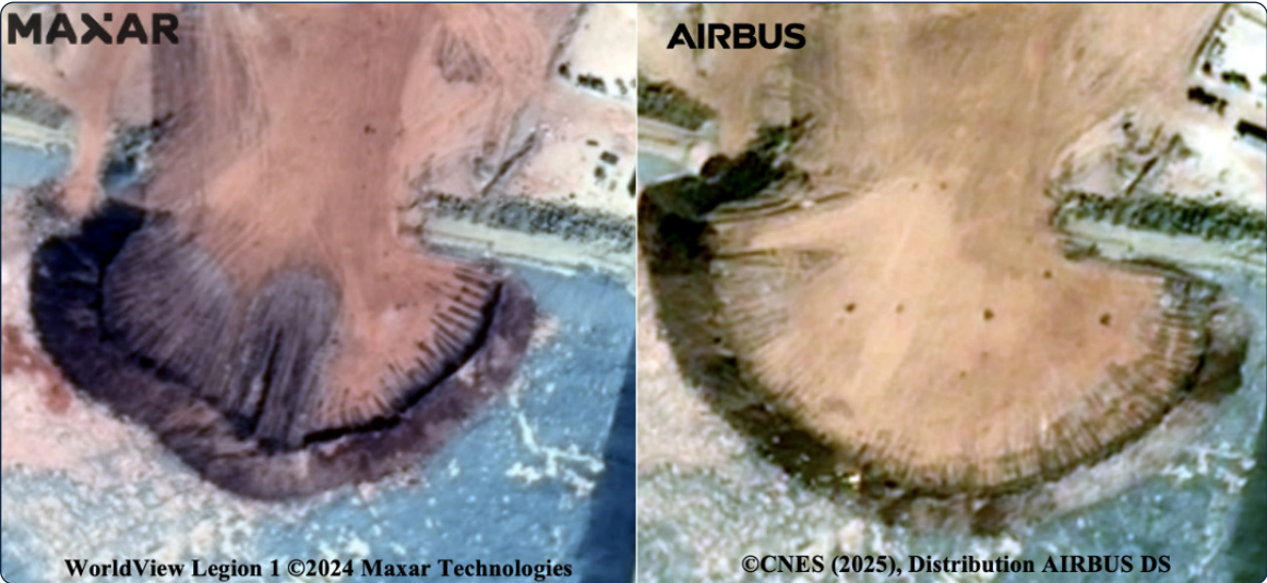
Figure 40: Satellite imagery of shifts in material along a curved containment area, possibly indicating the clearing, relocation, or expansion of ore or tailing storage, at Orshab, November 2024 (left) and January 2025 (right). The overall volume and surface texture of the deposit appear visibly altered.
