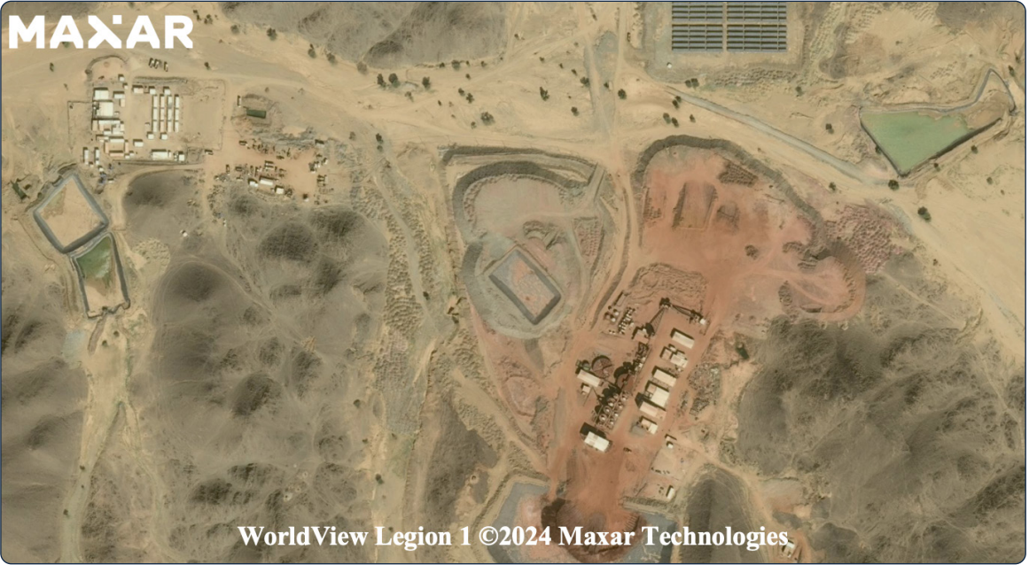
Figure 39: Satellite imagery of the Orshab site, November 2024. The site is located in Sudan's Red Sea State. The site has a large open-pit mine that is surrounded by ore and tailings piles. The southeast portion of the site contains an area for refining using the carbon-in-leach process.
