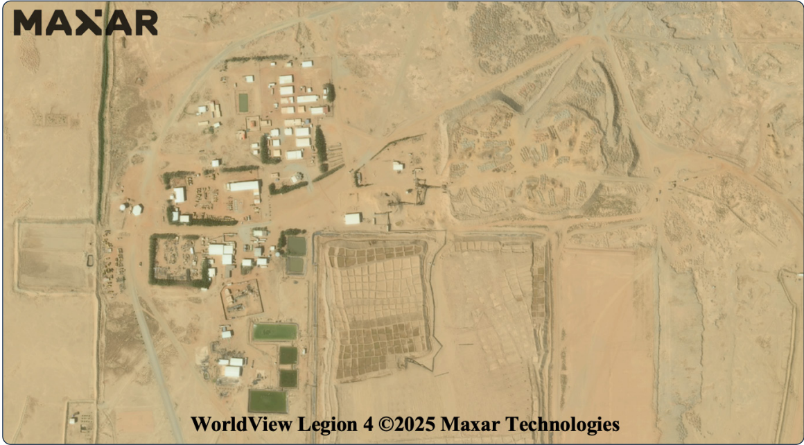
Figure 32: Satellite imagery of the Omdurman Mining site, March 2025. The site is located in Sudan's River Nile State. The site has a large open-pit mine with ore heaps and tailings mounds scattered nearby. A location for refining is located in the south, with a single leach heap draining into smaller ponds.
