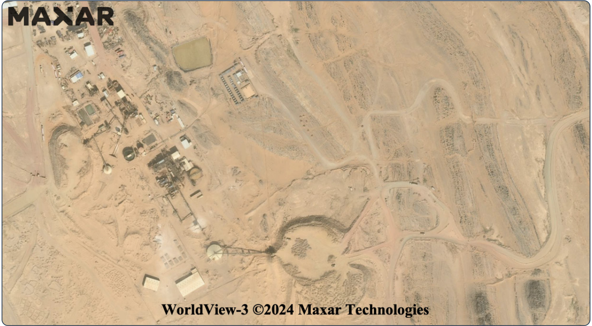
Figure 24: Satellite imagery of the Manub for Mining site, November 2024. The site is located in Sudan's River Nile State. The site has a series of small, open-pit mines, each with its own heaps and tailings mounds, along with a central area for refining that contains several holding ponds, leach heaps, chemical tanks, and leach ponds
